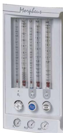
It has the function to regulate the capacity and the concentration of gas mixture (Air, O<sub>2</sub>, N<sub>2</sub>O) as well as to deliver it to the anaesthetic gas vaporizer.
