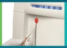
Due to its automatic retractable and self-wiping fill port, can aspirate whole blood, serum, urine, or other biological substance from syringe, tube or
