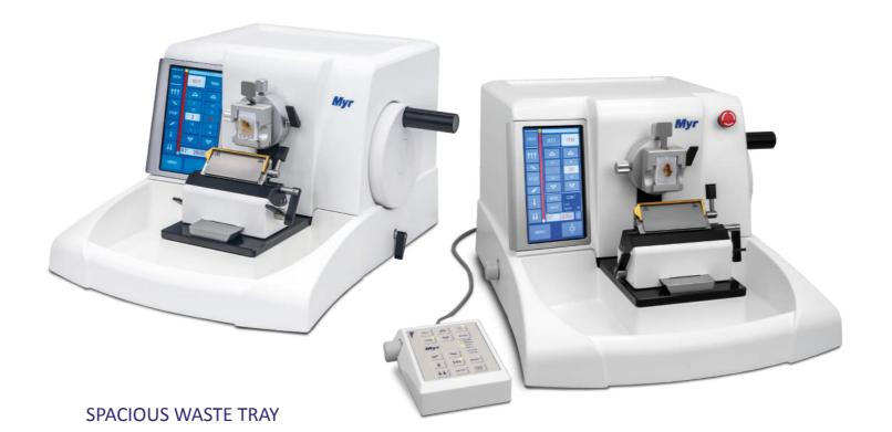
High volume waste tray (1.7 Liters) with special antistatic coating that prevents paraffin adhesion and minimizes the cleaning time. Additional design includes a surface for arm rest and an area on the top of the instrument for tool storage.
