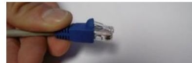
Slide boot back over lock clip
