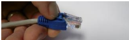
Pull boot back to access lock clip
