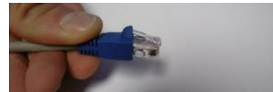
Slide boot back over lock clip
