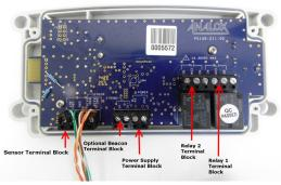
The Central Display's terminal blocks must be connected to the power supply, sensor, beacon and relays (if required).
