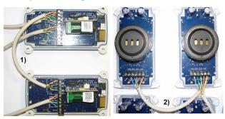
Daisy-chaining is the means by which the alarms can be connected sequentially. Follow the same wiring sequence described in step 5. Note that wiring access is on the rear of the unit only. The wiring can either be connected via the 'knock-out' on the rear of the unit or the optional gland(s) (Blanking discs to be removed) on the bottom of the unit.
