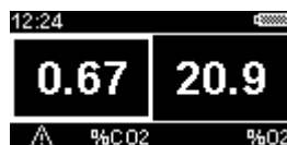
Figure 5 The main gas display showing that carbon dioxide levels have triggered an alarm
