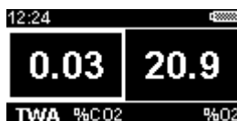
Figure 7 The main gas display showing the user has exceeded their TWA exposure to carbon dioxide.
