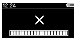
Figure 14 Oxygen fresh air calibration failed
