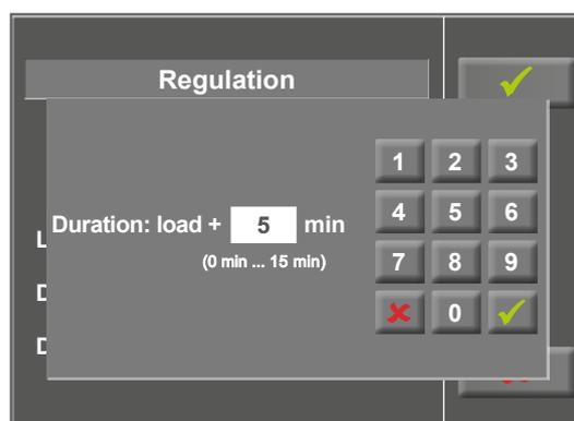
Figure 7-76: Setup – regulation method, screen 2
