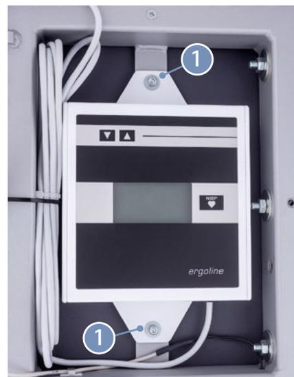
Figure 4-15: Control terminal under the couch surface
