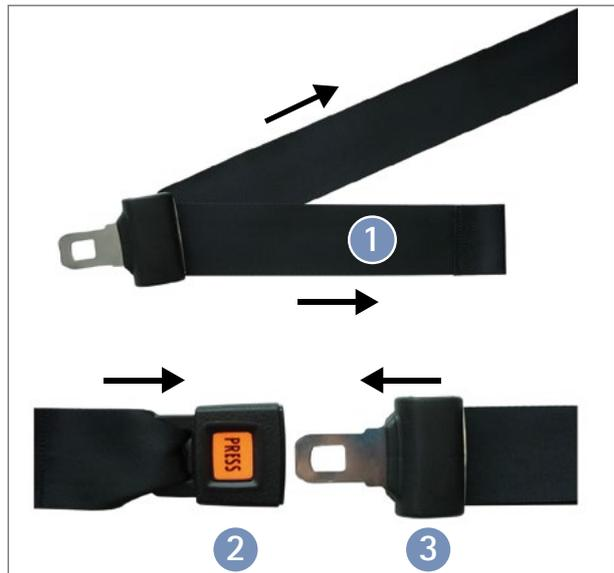
Figure 10-5: Adjusting and closing the safety belt
