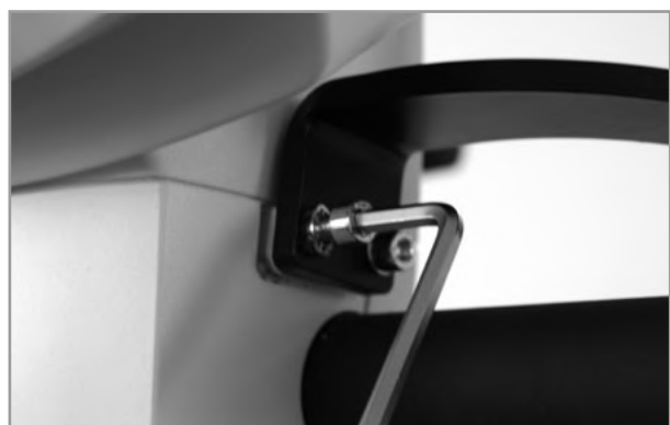
Figure 4-7: Mounting the leadwire holder
