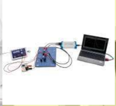
CHARGING & DISCHARGING COIL EXPERIMENT
