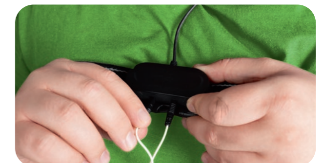
Respiratory effort and body position sensor is attached to the chest inductive belt
